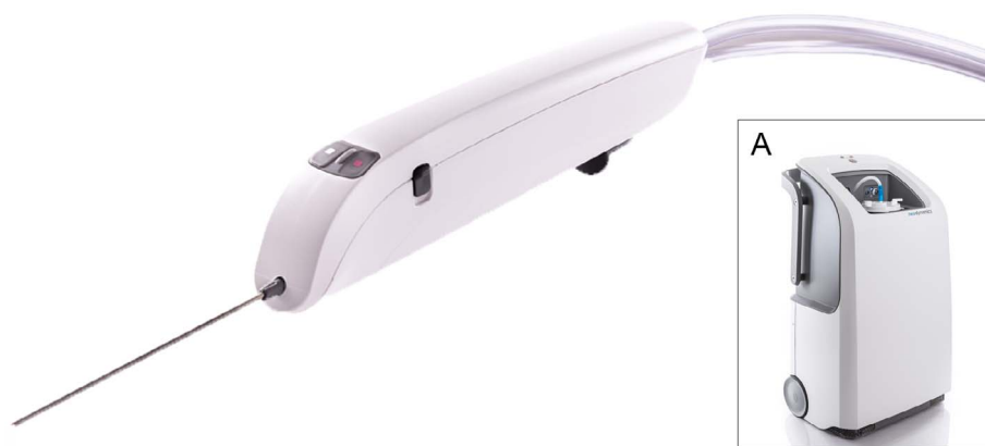
Fig. 5. Image of the NeoNavia biopsy device and base unit (A). The lever on the bottom of the device is used to extend the trocar and fixate it to the sampling needle with an internal spring mechanism. This is done when preparing the device for sampling to enable a sharp dissection tip while blocking the needle tip to keep healthy tissue from entering the sampling needle. The trocar retraction buttons on each side of the handle are used to retract the trocar, which allows sampling to start by unblocking the needle tip and initiating vacuum suction capability through the sampling needle. When the operator pushes the pulse button on top of the device a pneumatic pulse is activated which results in a forward movement of the biopsy needle. After filling the sampling needle with an adequate amount of tissue by moving the sampling needle through the suspicious lesion using pneumatic pulses, the sample is cut using the cutting button. Pushing the button initiates a rotational motion that separates the tissue inside the sampling needle from sur-
